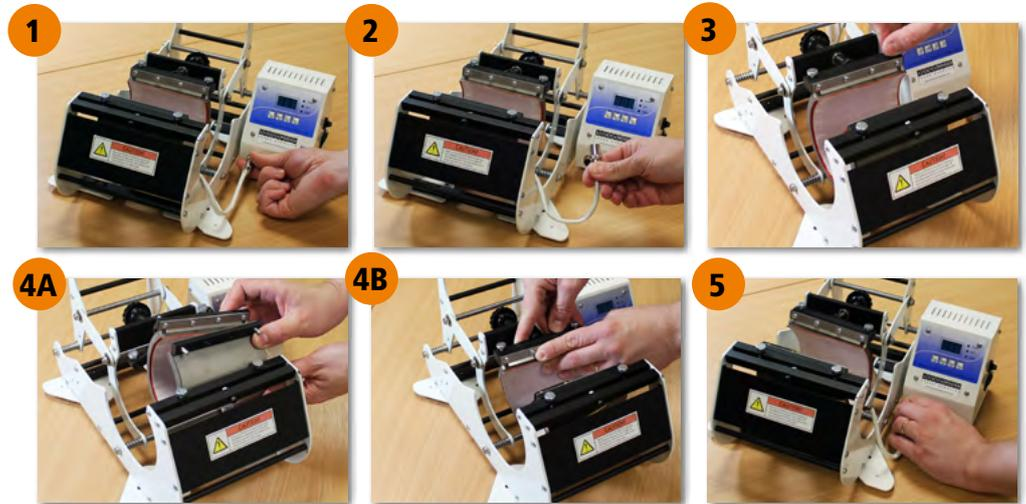
Before changing heater bands make sure that the press is unplugged from the mains and the machine is cool.
